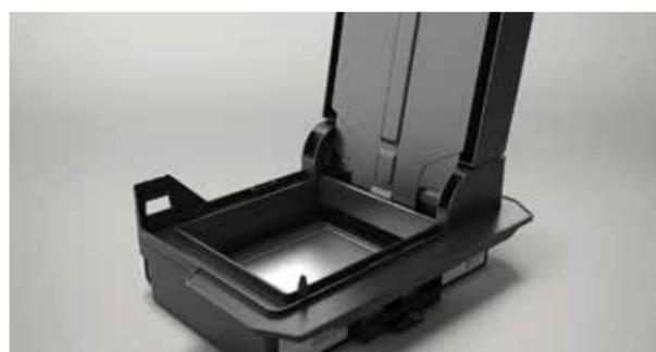
Depending on the type and number of objects intended for a print process, the Primeprint system dispenses the appropriate amount of print resin from the cartridge into the print vat and monitors its use. The software detects the fill level automatically and notifies the user when the material cartridge must be replaced.
