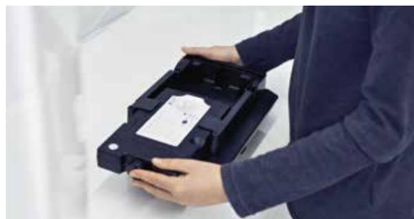
The Primeprint Material Unit consists of the vat and the insertion slot for the material cartridge. The material cartridge clicks into the material unit with a hand movement. Both the vat and the material cartridge are fitted with RFID tags. Once assembled, the software automatically pairs them and identifies them as a unit.
