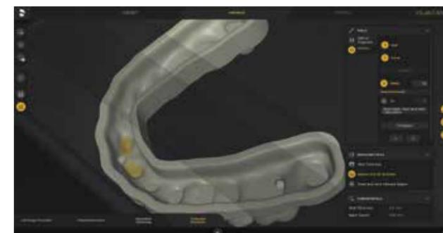
The software indicates where air may potentially get trapped during the wash process later on or where puddling of resin may occur, which might not be cleaned up. In this case, drainage canals can be positioned virtually, based on the planned print placement, directly in the CAM software without the need to go back to the design phase.
