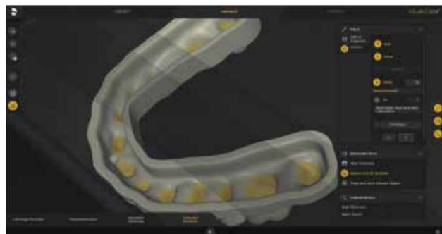
Support structures as well as drainage canals and vents are automatically placed by the software but can also be added, removed, and repositioned manually.
