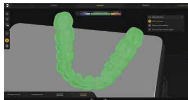
For quality enhancement, the software indicates compliance or noncompliance with manufacturer-specified wall strength – a special advantage of the validation process that was performed for each Primeprint material. As such, additional corrections can be made, for example in the case file when cases of noncompliance are detected.
