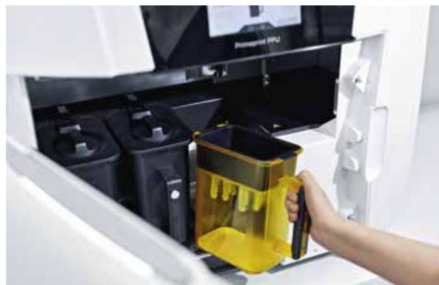
After the print is completed, only the Primeprint Box is removed from the printer and placed into the PPU. The Primeprint Box is sealed and protected from UV light; it does not require any additional contact precautions. Based on the RFID identifier, the individual job is detected and the fully automated post-processing begins with just one click on the screen. The rest is taken care of by the PPU.
