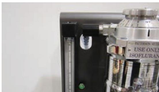
**STEP 7** Vaporizer should be positioned as shown with the tubing centered in the slots. Adjust if necessary.
