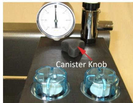
**STEP 3** Check inhalation/exhalation flutter disks. During shipping these disks MAY have come dislodged from their normal positions. They should be oriented flat on top of the valves beneath the dome caps as shown in the photo. If they are not as shown remove the dome caps, place the disks flat on the valves and replace the dome caps BEFORE using the anesthesia machine.
