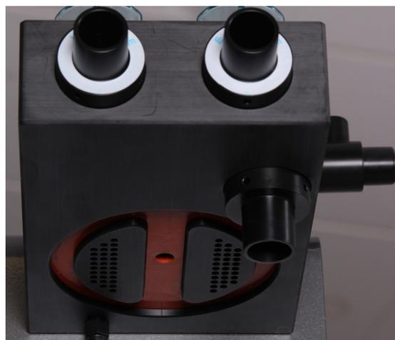
**STEP 4** Remove all CO<sub>2</sub> absorbent and remove as much dust as possible. Clean internal/external and divider sections of absorber canister with a mild soapy water solution. Pay specific attention to the top of canister where Sodasorb can build up. (Absorber Canister Replacement: 07-8935118)
