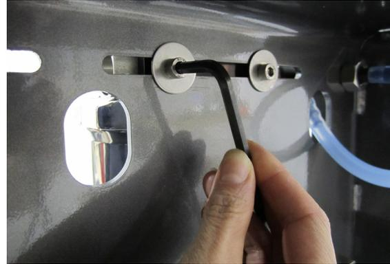
**STEP 9** Tighten drain stem as shown.
