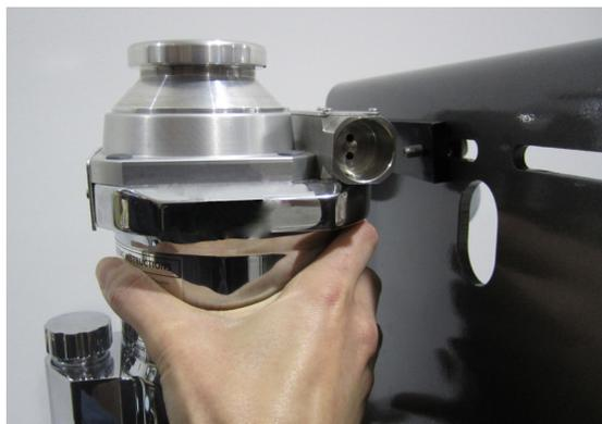
**STEP 6** Install female endcap onto the inlet side of vaporizer manifold. Install male endcap onto the outlet side of the vaporizer manifold.
